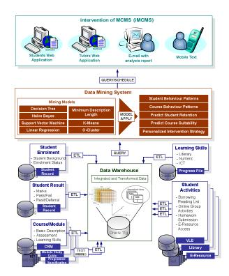
Figure 3. MCMS System Architecture
