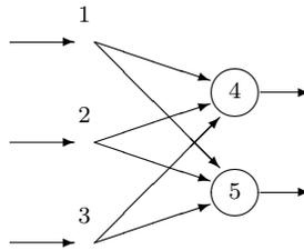
**Input** nodes of the network (nodes 1, 2 and 3) are associated with the input variables  $(x_1, \dots, x_m)$ . They do not compute anything, but simply pass the values to the processing nodes.
