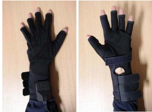
Figure 5. The 5DT data glove
