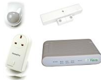
Figure 6: ZWave equipment. Clockwise, from top left: PIR, door switch, dimmer, control box.
