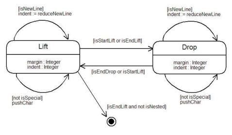
Figure 15.2.: Lift and Drop Mechanism
